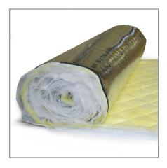
This Noise Barrier consists of flexible Mass Loaded Vinyl Barrier laminated to a quilted fiberglass decoupler on one side.
