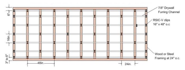
Framing at 16" OC: RSIC-V Value Clips at 16" x 48" OC 3 Layers of 5/8" Gypsum Board
