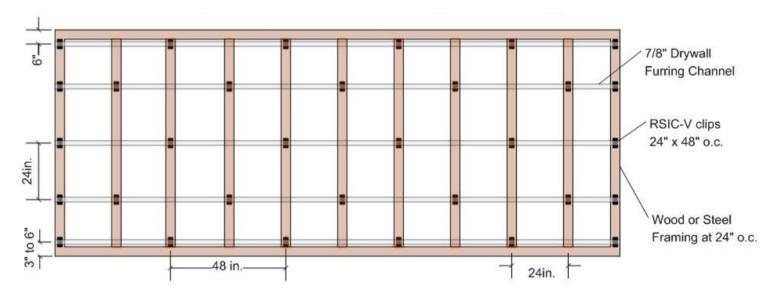
Framing at 16" OC: RSIC-V Value Clips at 24" x 48" OC with 1 or 2 Layers of 5/8" Gypsum Board
