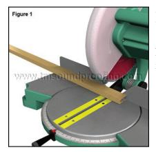
Once you have you determine the size needed, if necessary, trim your door bottom. Use a chop saw or table saw to create a perfectly straight cut.
